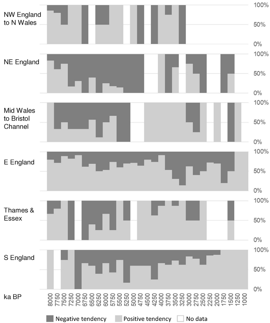
Fig. 8. Proportion of negative and positive sea-level tendencies within each 250 year interval for regional groups; NW England to N Wales (regions 30, 32, 33,34, 35), NE England (23, 24, 25, 26), Mid Wales to Bristol Channel (36, 43,44,45), E England (27, 37, 37, 39, 40, 41, 42), Thames & Essex (46, 47), S England (48, 49, 50, 51, 52, 53). Age labels indicate upper limit of the 250 year class. Index points assigned by their median age with no consideration of their 95% age range.
